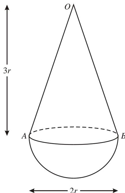
A child's toy consists of a uniform solid hemisphere, of mass  $M$  and base radius  $r$ , joined to a uniform solid right circular cone of mass  $m$ , where  $2m < M$ . The cone has vertex  $O$ , base radius  $r$  and height  $3r$ . Its plane face, with diameter  $AB$ , coincides with the plane face of the hemisphere, as shown in the diagram above.
