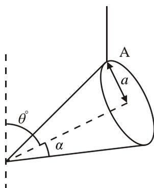
A uniform solid right circular cone has base radius  $a$  and semi-vertical angle  $\alpha$ , where  $\tan \alpha = \frac{1}{3}$ . The cone is freely suspended by a string attached at a point  $A$  on the rim of its base, and hangs in equilibrium with its axis of symmetry making an angle of  $\theta^\circ$  with the upward vertical, as shown in the diagram above.
