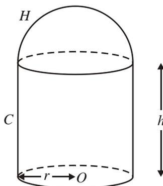
A body consists of a uniform solid circular cylinder  $C$ , together with a uniform solid hemisphere  $H$  which is attached to  $C$ . The plane face of  $H$  coincides with the upper plane face of  $C$ , as shown in the figure above. The cylinder  $C$  has base radius  $r$ , height  $h$  and mass  $3M$ . The mass of  $H$  is  $2M$ . The point  $O$  is the centre of the base of  $C$ .
