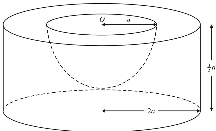
A uniform solid cylinder has radius  $2a$  and height  $\frac{3}{2}a$ . A hemisphere of radius  $a$  is removed from the cylinder. The plane face of the hemisphere coincides with the upper plane face of the cylinder, and the centre  $O$  of the hemisphere is also the centre of this plane face, as shown in the diagram above. The remaining solid is  $S$ .
